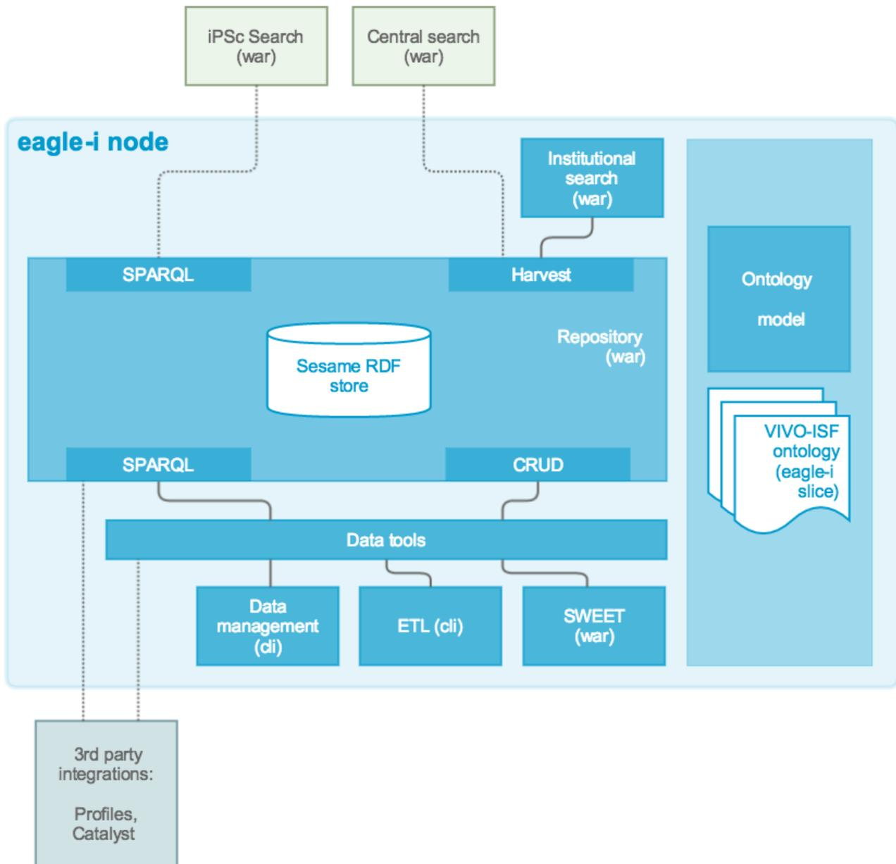
**Figure 2. Details of the eagle-i stack**
